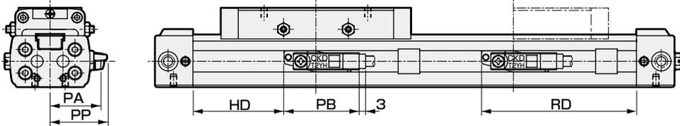
● 带气缸开关SRL3-G-\*\*\*-\*\*\*-\*\*\*-T\*\*V(T\*\*W, T\*\*Y)
