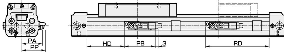
● 带气缸开关SRL3-※※-※※-※※※※-T※V(T※W, T※Y)
