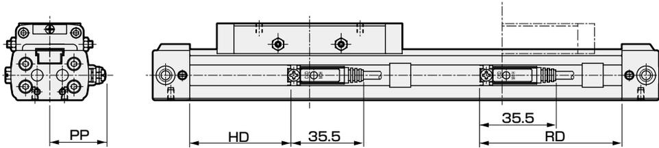
● 带气缸开关SRL3-G-\*\*\*-\*\*\*-\*\*\*-T\*\*H(T\*\*W, T\*\*Y, T2YD)
