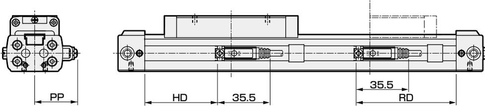
● 带气缸开关SRL3-※※-※※-※※※※-T※H(T※W, T※Y, T2YD)
