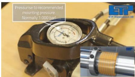
**6.** Open the pressure-reducing valve at the pump.
