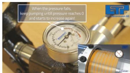
**4.** Open the pressure-reducing valve at the pump. (The pressure in the hoses falls).
