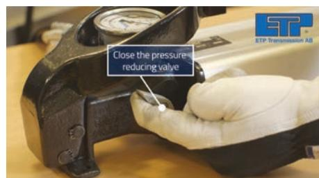
**5b.** Pressurise to recommended mounting pressure, which should be held for approx. 5-10 seconds.
