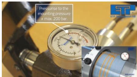
**3c.** Observe the pressure gauge. When the pressure suddenly falls, (the piston inside ETP-HYLOC has now started to move), continue to pump until the pressure has become 0 and starts to increase again. The piston inside ETP-HYLOC has now been moved to its end position.
