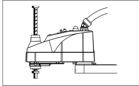
The height of Joint #3 (shaft) depends on manipulator model.
