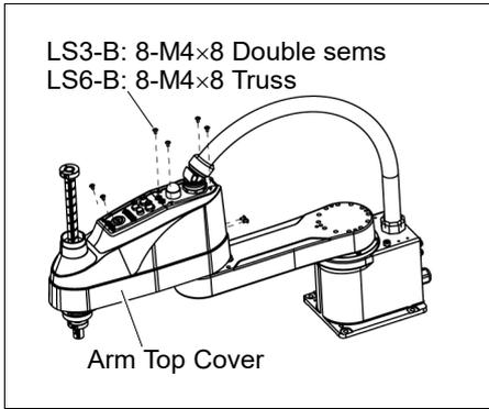
**Arm Top Cover Installation**    Put the arm top cover to the arm and secure with the Arm Top Cover mounting bolts. After securing the Arm Top Cover, make sure that the lower limit mechanical stop is not touching the cylindrical part of the Arm Top Cover.
