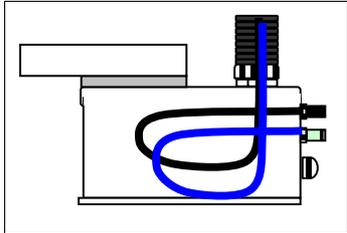
Put the air tube along the left side wall as shown in the picture.
