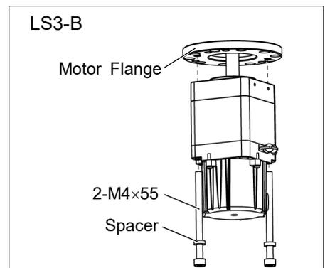
Joint #2 Motor Installation
