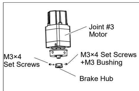
Joint #3 brake Installation (1) Mount the brake to the brake plate.
