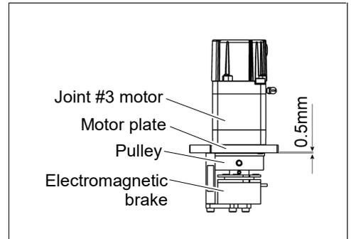
Tighten one of the set screws vertically on the flat face of the motor shaft.
