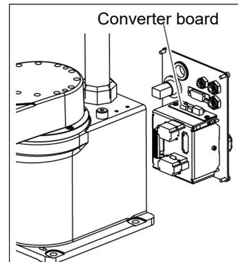
(4) Remove the converter board from the mount base.
