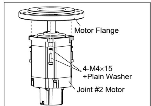
Joint #2 Motor Installation
