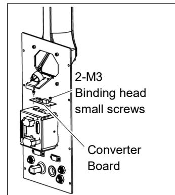
Converter board (1) Mount the converter board on the mount base.
