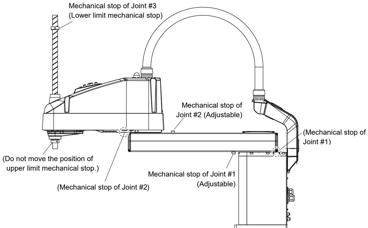
**5.2.1 Setting the Mechanical Stops of Joints #1 and #2**
