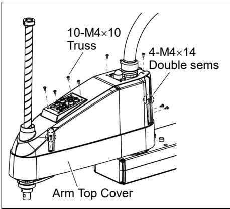
**Arm Top Cover Installation**    Put the arm top cover to the arm and secure with the Arm Top Cover mounting bolts. After securing the Arm Top Cover, make sure that the lower limit mechanical stop is not touching the cylindrical part of the Arm Top Cover.
