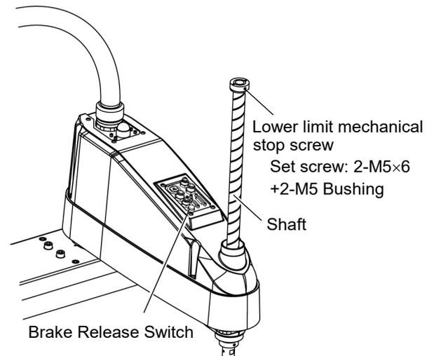
When you press the brake release switch, the shaft may lower or rotate due to the weight of the end effector. Be sure to hold the shaft by hand while pressing the button.
