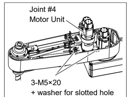
If the unit is tilted, the belt will not have the proper tension.
