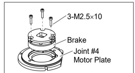
Joint #4 Brake Installation
