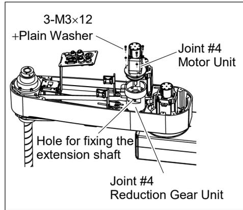
(10) Remove Joint #4 motor unit from the reduction gear unit.
