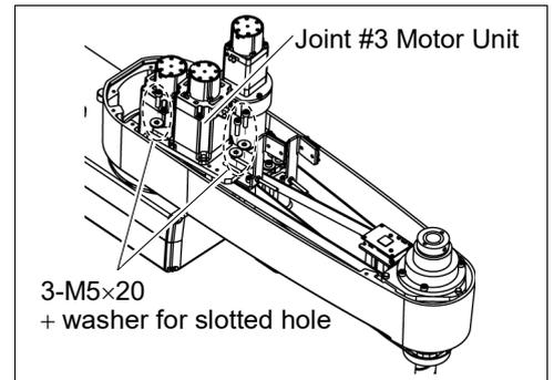
If the unit is tilted, the belt will not have the proper tension.
