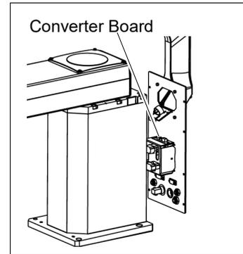
(4) Remove the converter board from the mount base.
