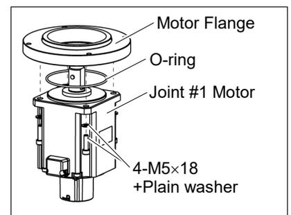
Joint #1 motor Installation
