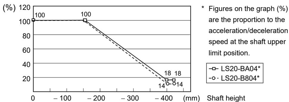
\* Figures on the graph (%) are the proportion to the acceleration/deceleration speed at the shaft upper limit position.
