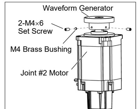
Joint #2 Motor Installation
