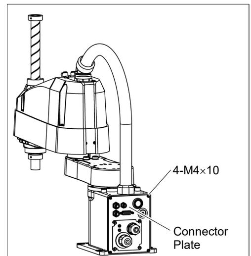
When mounting the Connector Plate, be careful of the following.
