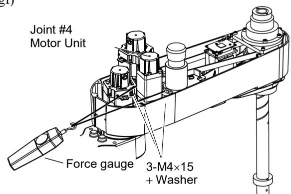
NOTE To check belt tension with the tension meter, refer to *Maintenance: 8.4 Checking the Timing Belt Tension (U1, U2 Belt)*.
