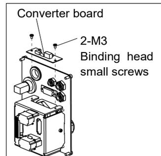
(2) Connect the connectors to the converter board.
