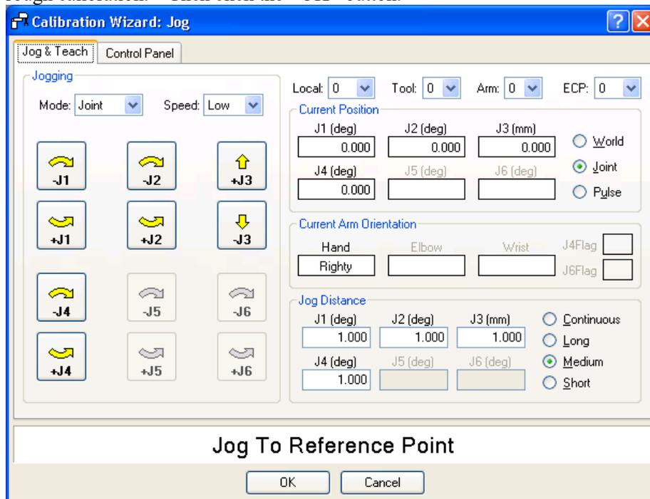
\* Position Joint #2 only and move Joint #3 to around 0 pulse.
