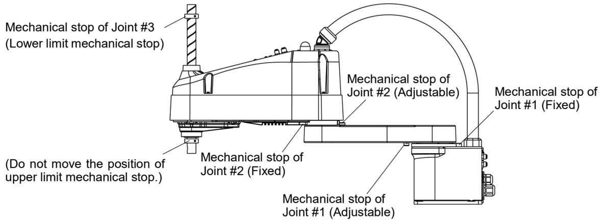
**5.2.1 Setting the Mechanical Stops of Joints #1 and #2**
