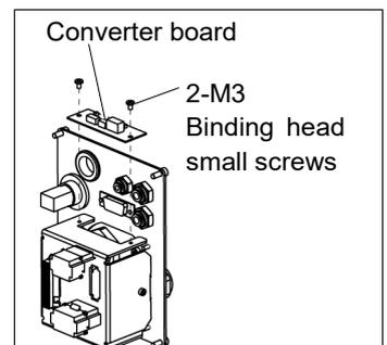
Converter board (1) Mount the converter board on the mount base.
