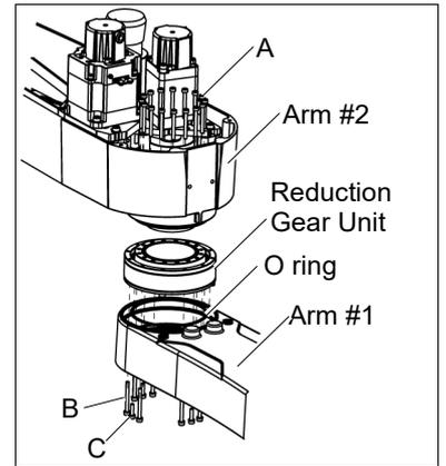
Loosely secure all bolts in a crisscross pattern so that the bolts will be secured evenly. Then, using a torque wrench, tighten each bolt securely in a crisscross pattern at the torque specified in the table below.
