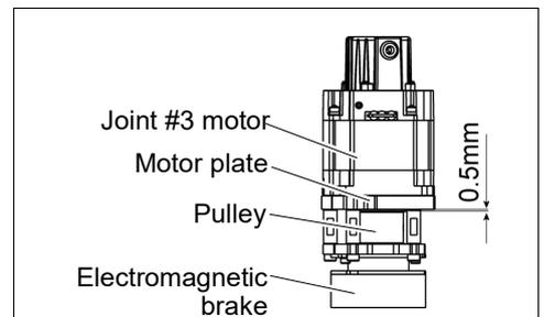
When the brake disc is not aligned, manually adjust the position by following the steps below.
