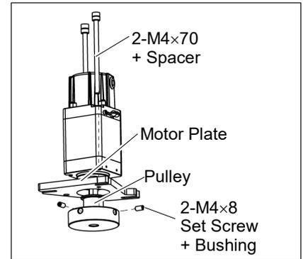
Be sure to fit the end face of the pulley to the end face of the motor shaft.
