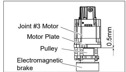
Tighten one of the set screws vertically on the flat face of the motor shaft.
