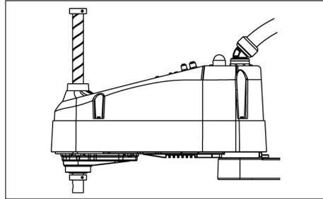
The height of Joint #3 depends on manipulator model.
