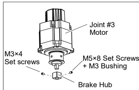
Joint #3 brake Installation (1) Mount the brake to the brake plate.
