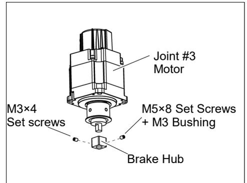
(3) Mount the Joint #3 motor to the motor plate while aligning the hub to the brake disc.
