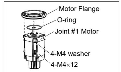
Joint #1 motor Installation
