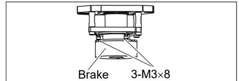
(2) Mount the brake hub to the pulley of the Joint #3 motor.
