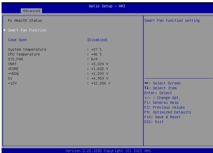
This section displays the system's health information, i.e. voltage readings, CPU and system temperatures, and fan speed readings
