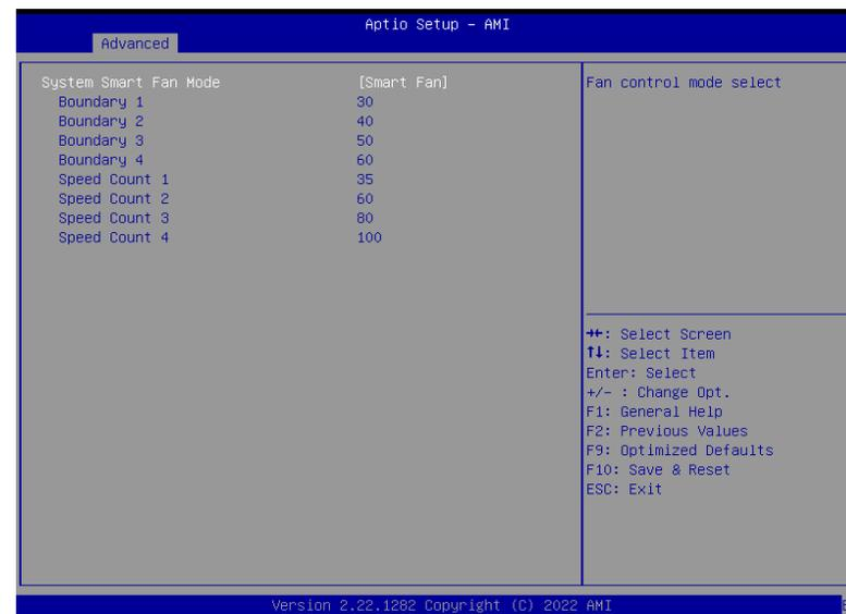
Smart Fan is a fan speed moderation strategy dependent on the current system temperature. When the system temperature goes higher than the Boundary setting, the fan speed will be turned up to the setting of the Fan Speed Count that bears the same index as the Boundary field.
