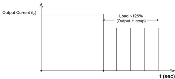
It is not recommended to prolong the duration of  $I_o$  when it is <125% but >100%, since it may cause damage to the PSU.
