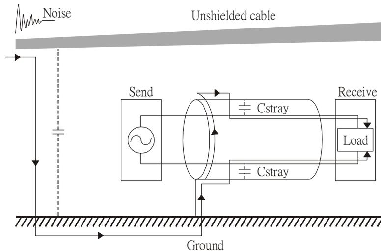
5. When excessive pulse modulated currents pass through an un-grounded AC drive cable, it acts as an antenna and creates radiated interference.
