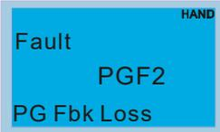
A blue rectangular display showing the text "Fault", "PGF2", and "PG Fbk Loss" in white. A small "HAND" icon is in the top right corner.      | PG feedback loss<br><br><u>corrective action</u><br>Check the PG feedback wiring.                                                                                                                                                                                                               |
