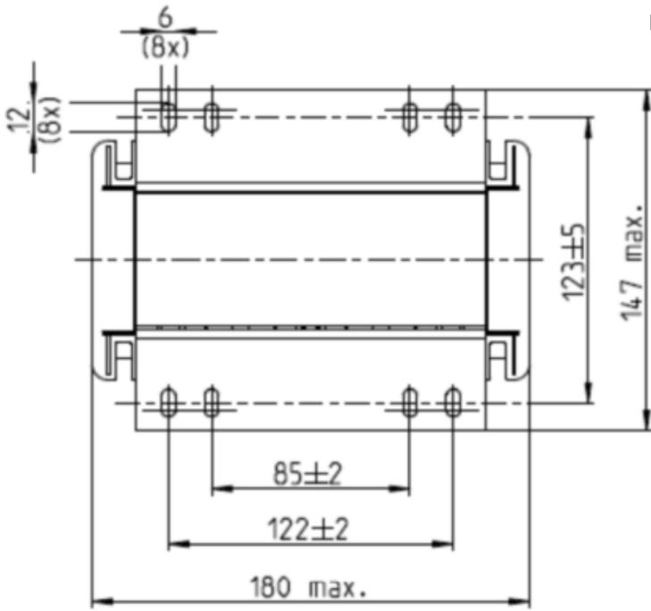
Installing screw: M6
