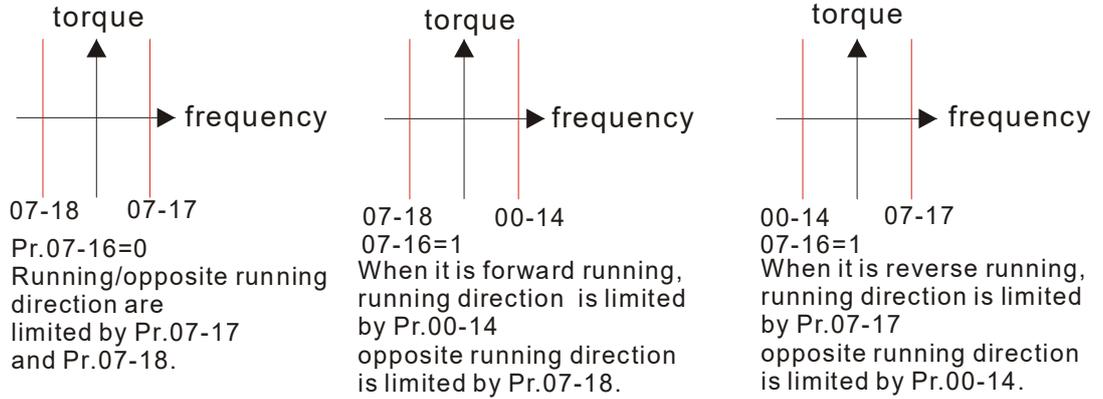
**07-17** Torque Mode + Speed Limit
