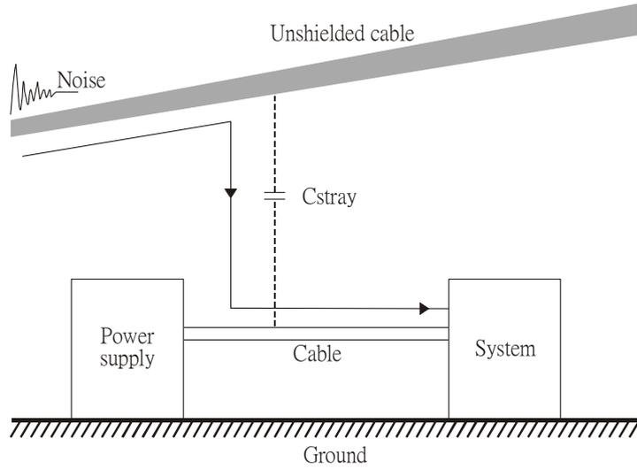
3. Common-mode noise is coupled via the power cable to other power systems then the cable of such a power system is coupled to the transmission system, as shown in Figure 3.
