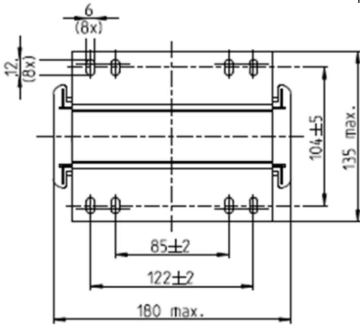
Installing screw: M6
