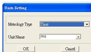
Choose the **Metrology Type** and the **Unit Name**. For **Metrology**, the choices are Length, Square Measure, Volume/Solid Measure, Weight, Speed, Time, and Temperature. The unit name changes automatically when you change metrology type.
