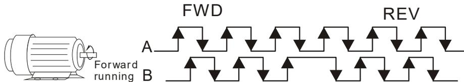
2: Phase B leads in a forward run command and phase A leads in a reverse run command
