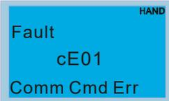
A blue rectangular display showing the text "Fault", "cE01", and "Comm Cmd Err" in white. A small "HAND" icon is in the top right corner.   | Illegal function code<br><br><u>corrective action</u><br>Check if the function code is correct (function code must be 03, 06, 10, 63).                                                                                                                                                          |
