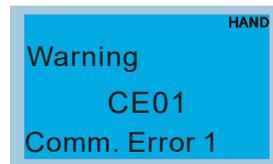
1. Press ENTER to RESET. If there is no response, contact your local distributor for instructions to return the equipment to the factory. To view the DC bus fault voltage value, output current and output voltage, press MENU and then choose Fault Record for details (refer to the descriptions in the above #4 Fault Record).
