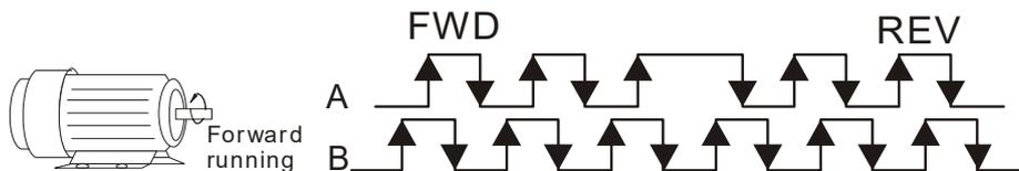
3: Phase A is a pulse input and phase B is a direction input. (low input=reverse direction, high input=forward direction)
