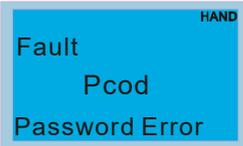
A blue rectangular display showing the text "Fault", "Pcod", and "Password Error" in white. A small "HAND" icon is in the top right corner. | Password error<br>After entering the wrong password three consecutive times, the keypad is locked.<br><br><u>corrective action</u><br>Refer to Pr.00-07 and Pr.00-08 settings for more information. Cycle the power for the motor drive to clear the lock and enter the correct password.       |
