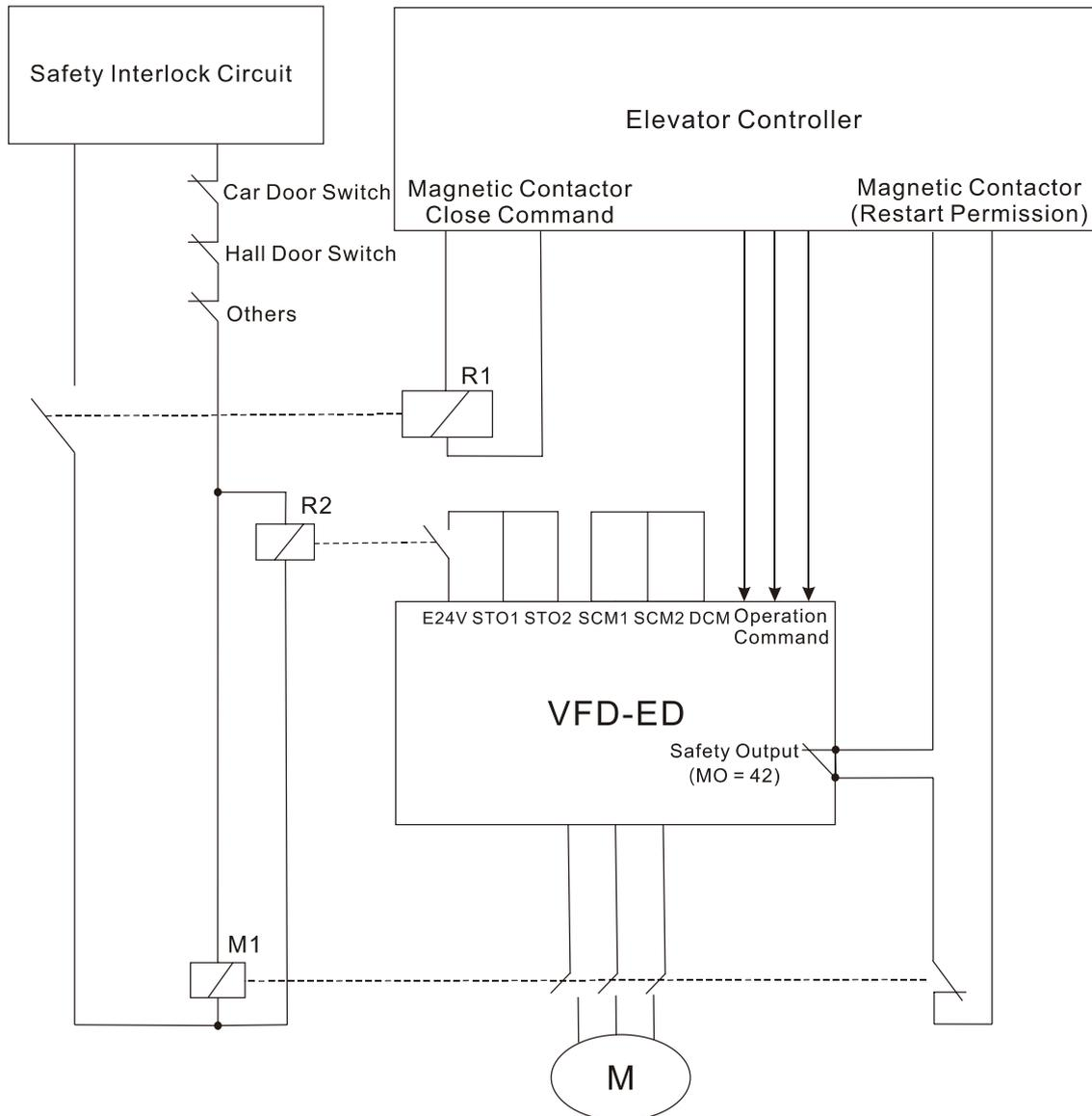
Note: "R" in R1/R2 stands for Relay; "M" in M1 stands for MC (Magnetic Contactor)
