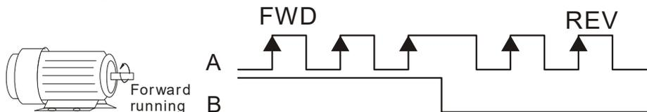
4: Phase A is a pulse input and phase B is a direction input. (low input=forward direction, high input=reverse direction)
