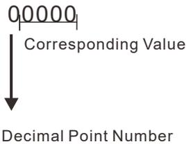
For example, if you use rpm to display the motor speed, and the corresponding value for the four-pole motor, 60 Hz is 1800. You can set this parameter to 1800 to indicate that the corresponding value for 60 Hz is 1800 rpm. If the unit is rps, set to 10300 to indicate that the corresponding value for 60 Hz is 30.0 (one decimal point).
