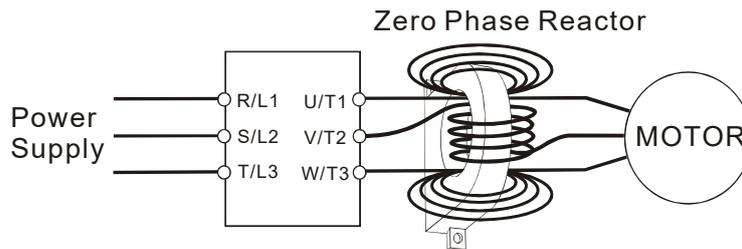
2. Place all wires through the middle of four zero-phase reactors without winding.
