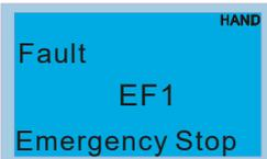
A blue rectangular display showing the text "Fault", "EF1", and "Emergency Stop" in white. A small "HAND" icon is in the top right corner.  | Emergency Stop<br>When you set the Multi-Function Input command (MI1–MI8) to #28 Emergency stop (EF1) (Motor coasts to stop), the motor drive stops running.<br><br><u>corrective action</u><br>Press RESET after you clear the fault.                                                          |
