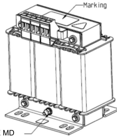
Tightening torque : 0.6–0.8 Nm
