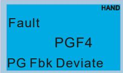
A blue rectangular display showing the text "Fault", "PGF4", and "PG Fbk Deviate" in white. A small "HAND" icon is in the top right corner.   | PG slip error<br><br><u>corrective action</u><br>1. Check the PG feedback wiring.<br>2. Check if the settings for PI gain and acceleration/deceleration are appropriate (Pr.10-07, Pr.10-08).<br>3. Contact the dealer or manufacturer to return the motor drive to the factory for repair.     |
