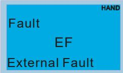
A blue rectangular display showing the text "Fault", "EF", and "External Fault" in white. A small "HAND" icon is in the top right corner.    | External Fault<br>When you set the Multi-Function Input command (MI1–MI8) to #10 EF input (Pr.07-28) and when multi-function input terminals are triggered to close, the motor drive stops running.<br><br><u>corrective action</u><br>Press RESET after you clear the fault.                   |
