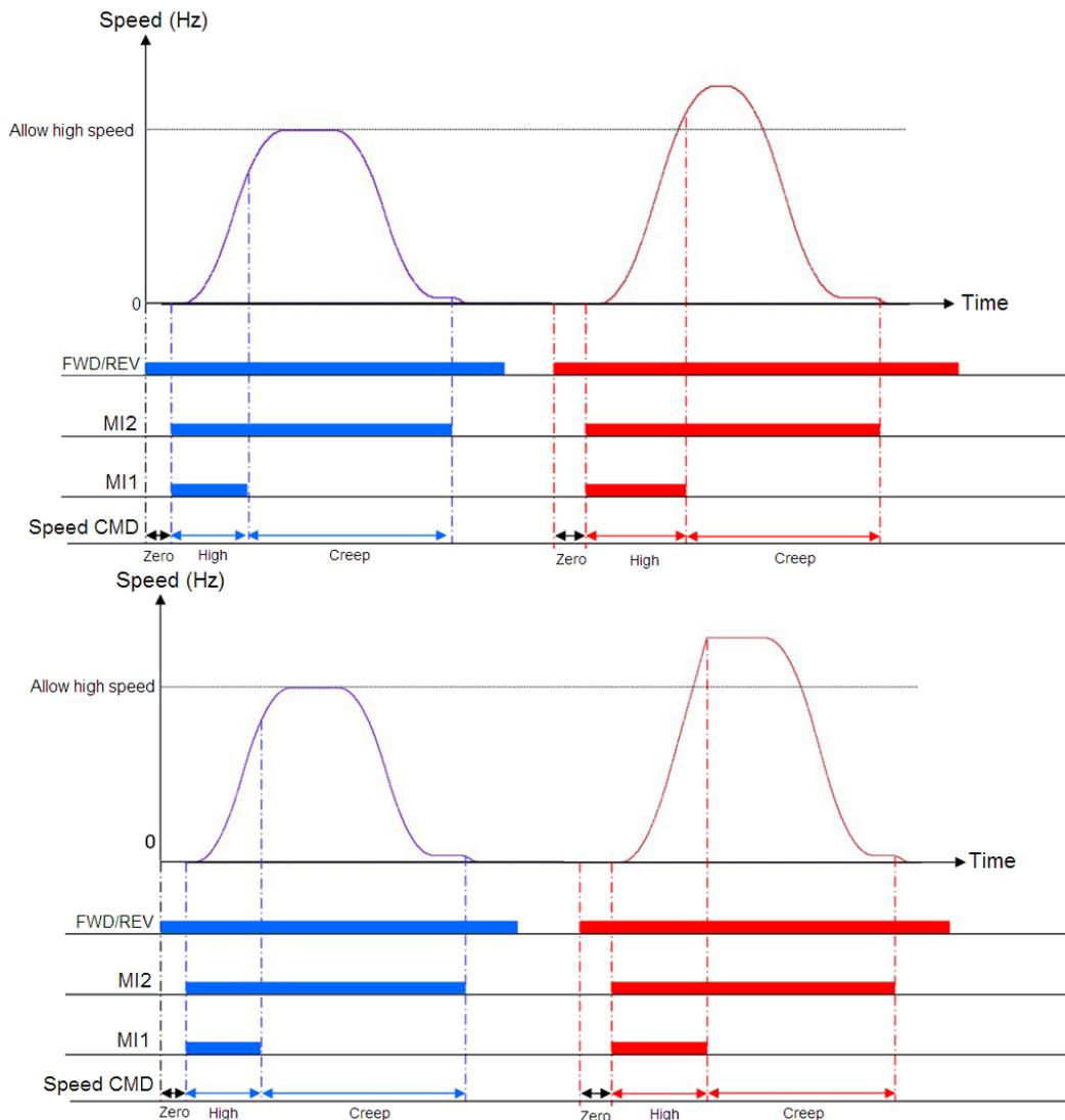
**Case 3. Deceleration point (instead of high speed) is given before allowed speed and high speed time is zero**
