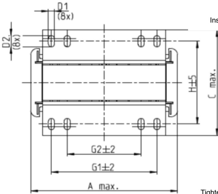
Installing screw: M5
