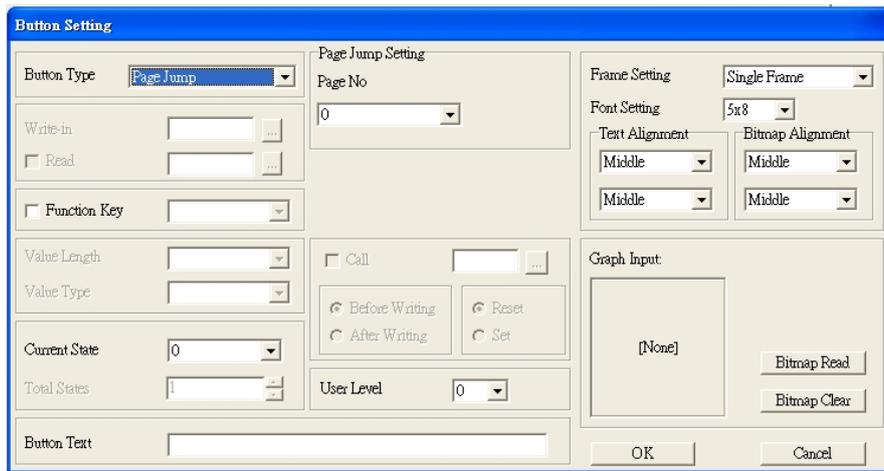
**Button Type:** specifies the button's functions. **Page Jump** and **Constant Setting** are the only functions currently supported.
