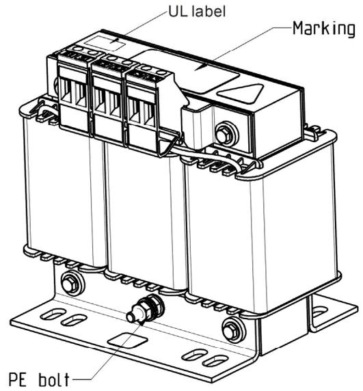
Tightening torque: 1.0–1.2 Nm
