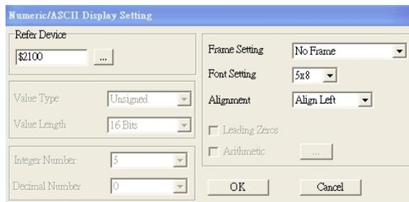
Click [...]. In the **Refer Device** dialog box, choose the VFD communication port that you need. If you want to read the output frequency (H), set the **Absolute Addr.** to 2202. For other values, refer to the ACMD Modbus Comm Address List in Pr.09-04 in Chapter 12.
