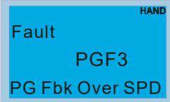
A blue rectangular display showing the text "Fault", "PGF3", and "PG Fbk Over SPD" in white. A small "HAND" icon is in the top right corner.  | PG feedback stall<br><br><u>corrective action</u><br>1. Check the PG feedback wiring.<br>2. Check if the settings for PI gain and acceleration/deceleration are appropriate (Pr.10-05, Pr.10-06).<br>3. Contact the dealer or manufacturer to return the motor drive to the factory for repair. |
