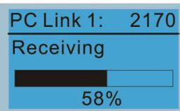
Start to upload parameters to VFDSOft.
