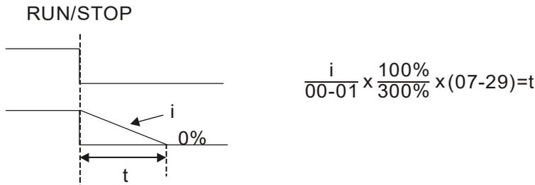
➤ **07-30** DC Brake Current Level at Stop
