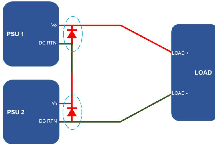
Fig. 30: Series connection with external reversed diode
