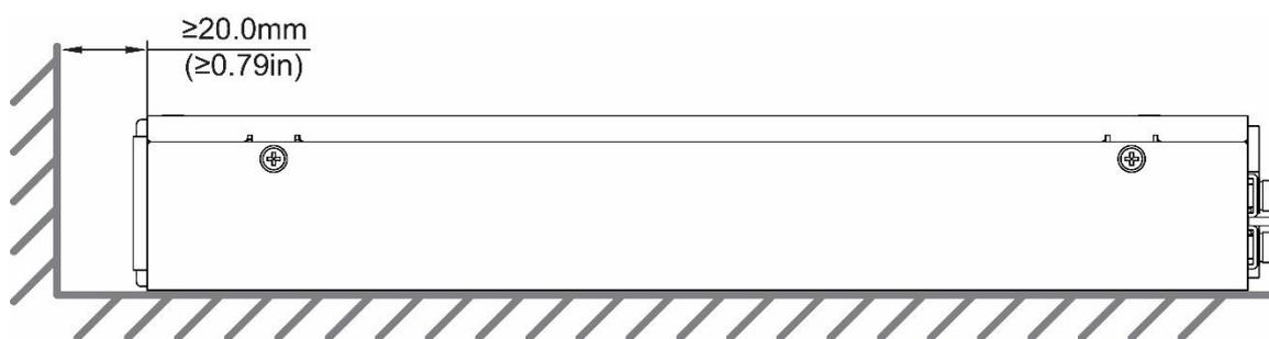
Fig. 2: Standard mounting orientation
