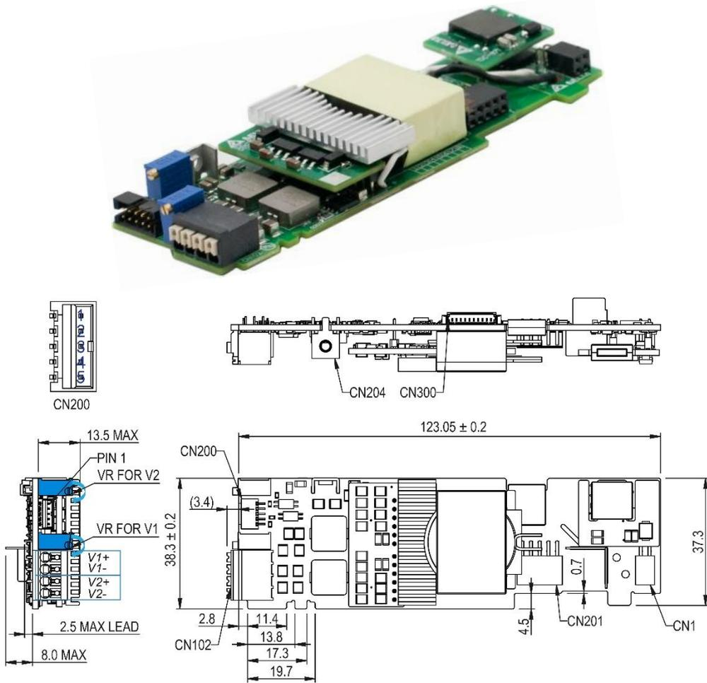
Fig. 8: Dimensional drawing Single Slot Dual Output Module
