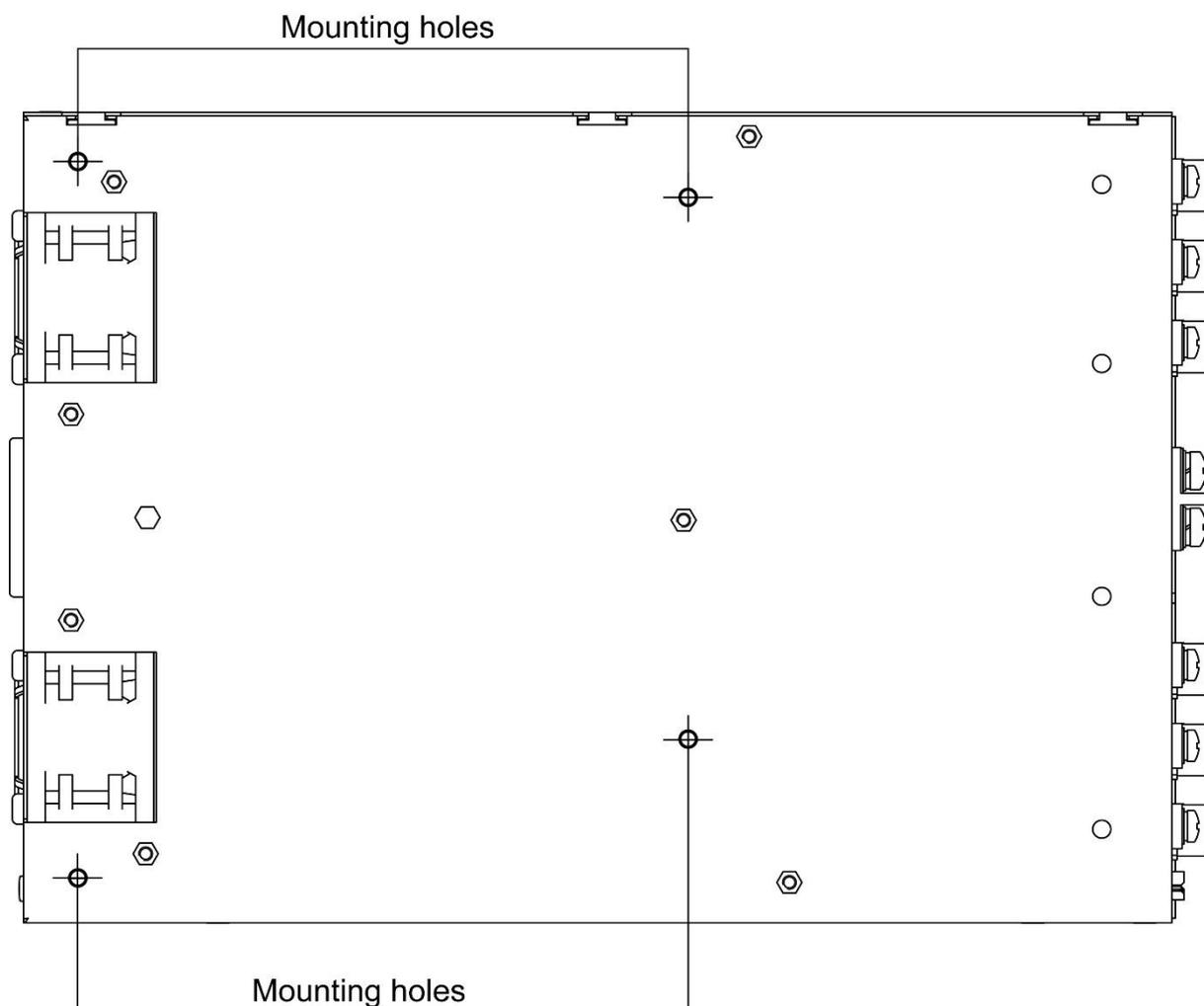
Fig. 4: Position of mounting holes
