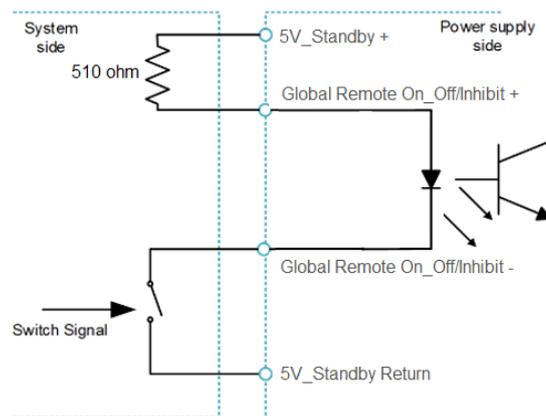
Fig. 31: Global Remote On\_off connection
