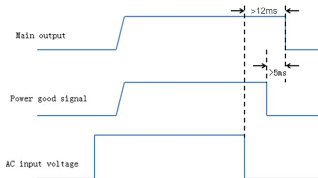
Fig. 26: Power good signal sequence
