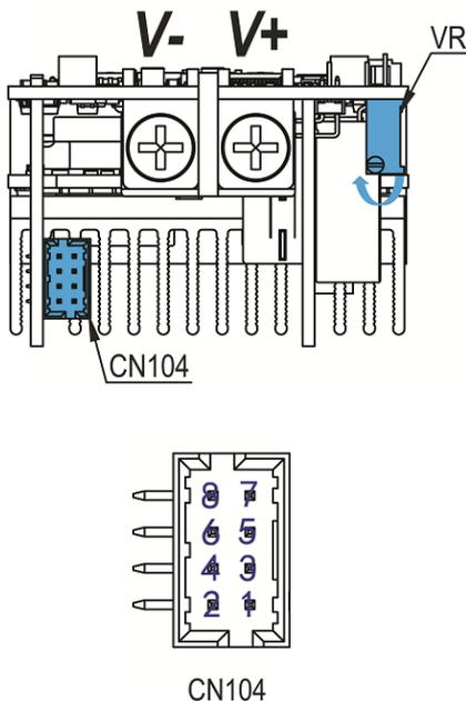
Fig. 16: -x2 Module connector
