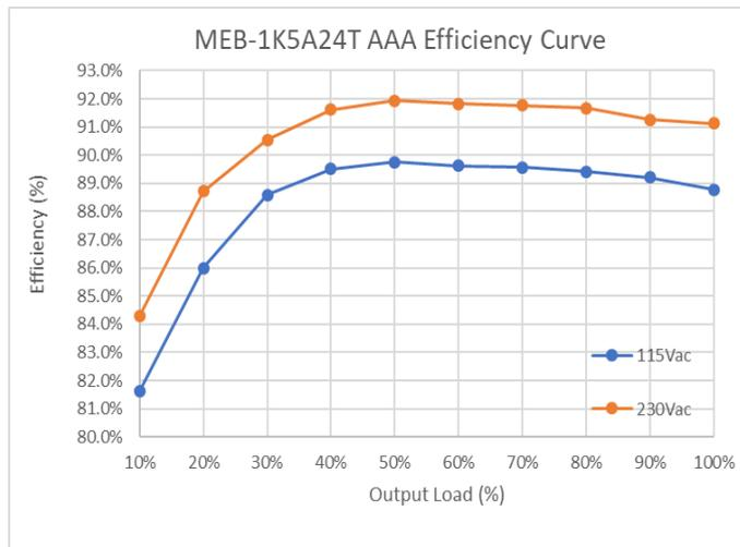
Figure 1-1. Typical efficiency Curve for MEB-1K5A24T AAA
