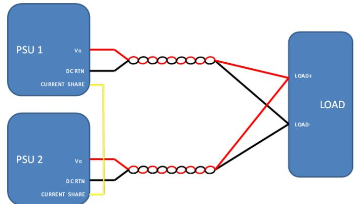
Fig. 10: Parallel connection
