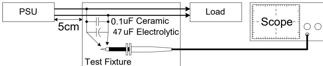
Figure 2. Ripple & Noise testing set up
