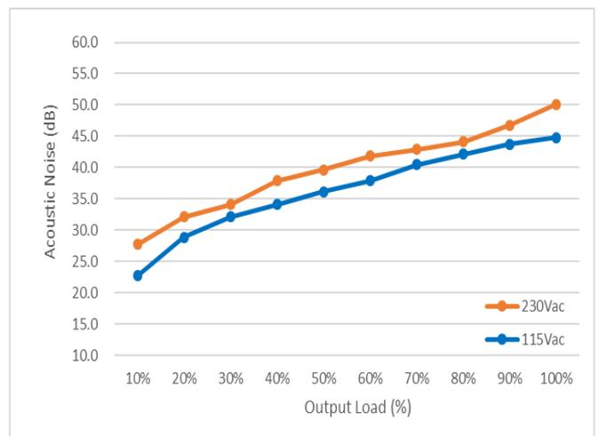
Figure 3-3. Typical acoustic noise curve for MEB-1K5A48T AAA
