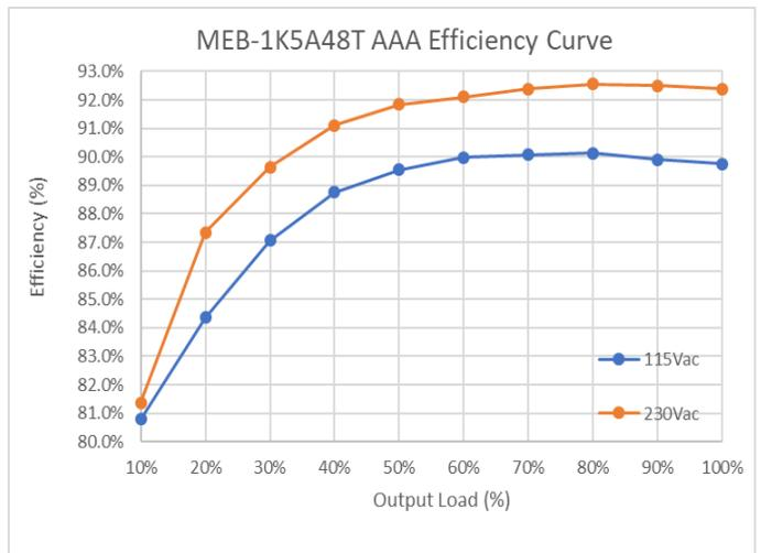
Figure 1-2. Typical efficiency Curve for MEB-1K5A48T AAA
