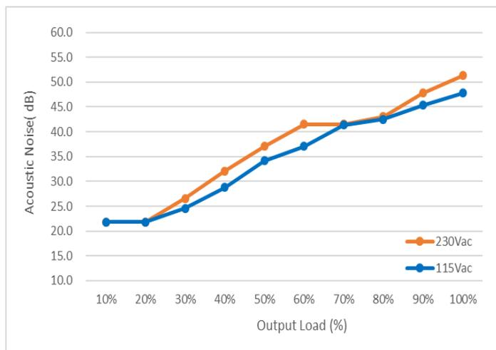
Figure 3-2. Typical acoustic noise curve for MEB-1K5A24T AAA
