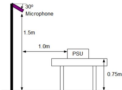
Figure 3-1. Acoustic noise testing set up
