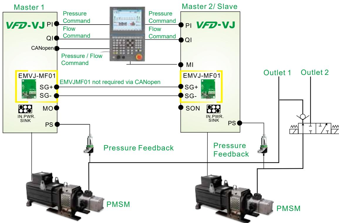
**Note 1 :** EMVJ-MF01 is not required for the Servo Drive VFD-VJ-C Series.
