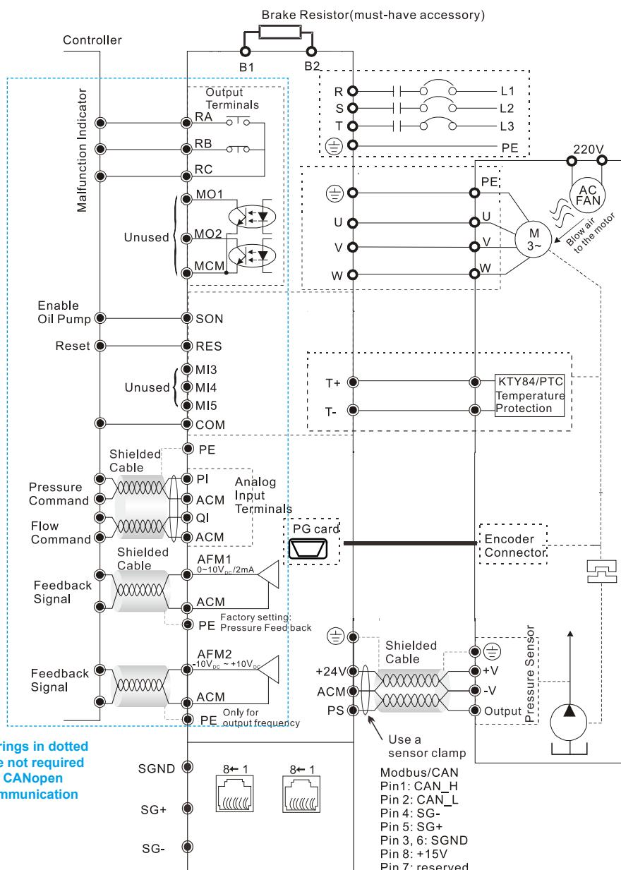
**\*Note 1 :** For HES063H43C ~ HES100H43C (Please wind the wire through the zero phase reactor at least 3 turns before connecting to the motor)
