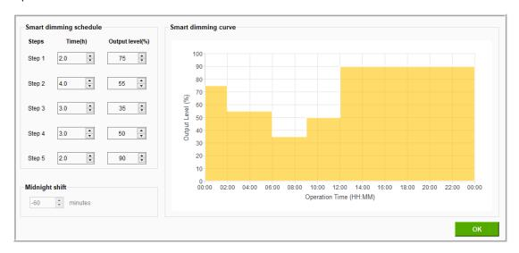
Note: When all steps are finished, the light level will remain in last level (level in step 5) for all three modes.
