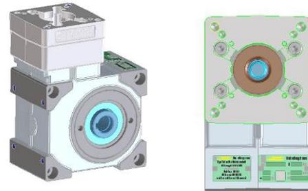
Screws should be tightend in severals steps across with defined torque according to table underneth.
