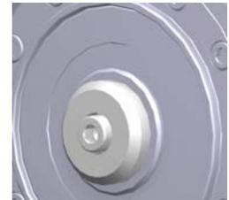
Mount retaining disk / lock screw and tighten
