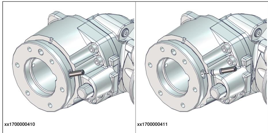
When calibrating axis 6, push in the calibration tool into the turning disc until the snap ring engages, no further.
