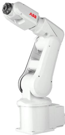
The IRB 120 robot is the latest addition to ABB's new fourth-generation of robotic technology. It is ideal for material handling and assembly applications and provides an agile, compact and lightweight solution with superior control and path accuracy.
