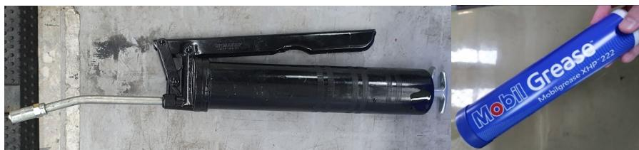
It is recommended to use Mobil SHC220 grease. The working temperature range of this grease is -40°C to 177°C
